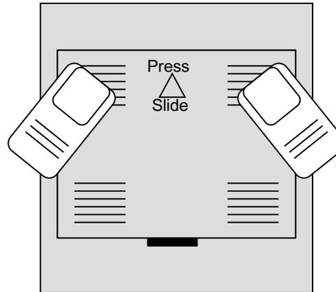
**Battery Installation** Uses three (3) AA batteries. Hold nFOCUS upside down with white adjustment knobs down. Insert arrowed end of access plate under lip of opening with arrow pointing down. Press down on access plate and slide upwards until securely attached.
